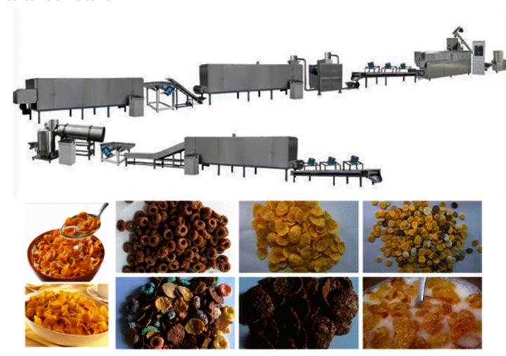
The above is the production process of cornflakes. The most important thing is the application of extrusion technology. The technology is also the technology that produces the highest use rate of cornflakes. The produced corn flakes are popular with consumers, in similar goods It is always in the level of sales.
