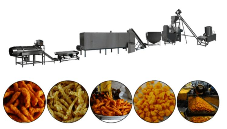
Kurkure making machine is a kind of production equipment for making new extruded small food that corn grits as the main raw material, which is extruded and twisted into a curly shape by two turntable production line is completed from raw material configuration, extrusion puffing, frying or baking, spr and flavoring to the finished product at one time. It can also produce different shapes of puffed food sandwich snack food and sandwich cookie, nutritious breakfast, corn flakes, etc.
