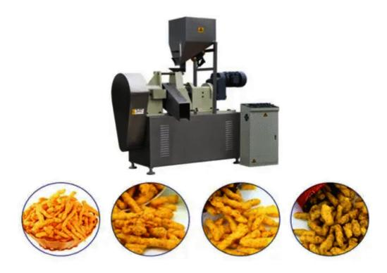
**Kurkure Production Line** consists of a mixer, screw conveyor, extruder, fryer elevator, flavoring drum, cooler, and packaging machine. The whole line is highly automated, which greatly saves time in the production process, improves work efficiency, and brings considerable economic benefits to food processing plants.
