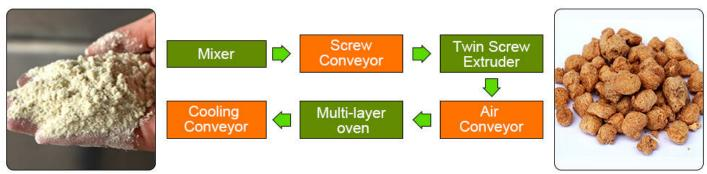
Mixer-Screw Conveyor-Twin Screw Extruder- Air Conveyor- Dryer- Hoister- Flavoring Machine
