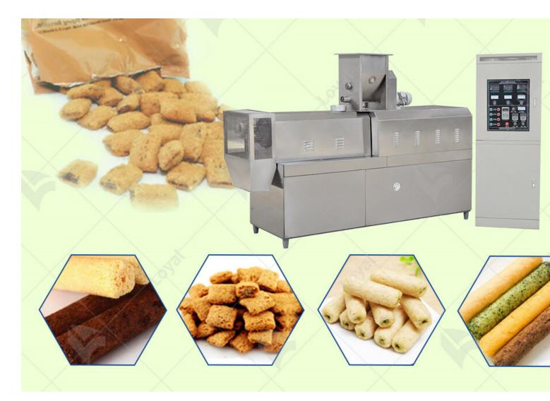
III. Twin - Screw Extruder: The Core Technology of Puffed Food
