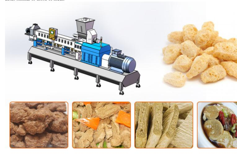
The whole Textured Soya Protein production line can automatically complete the production from m extruding, air conveyor, multi-layer oven, cooling conveyor to the finished product.
