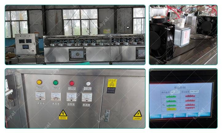
Detail of Industrial Tunnel Microwave Food Power Drying Sterilization Machine in production workshop
