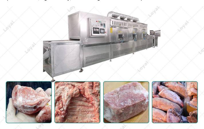
Application Of Tunnel Microwave Frozen Meat Mutton Processing Thawing Machine in Manufacturer What Is The Feature Of The Industrial Automatic Microwave Thawing Equipment?
