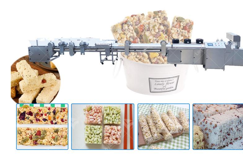
Mixer - screw conveyor- Twin-screw extruder-Air conveyor - drying machine - Hoister - double roller f machine - Cooing machine
