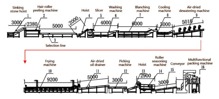
Flow Chart of Automatic Frozen French Fries Production Line Peeling -- Cutting -- Rinsing -- Blanching -- Shaken And Drained -- Frying -- Deoiling-- Seasoning --Freezing -- Weighing and Packing.Flow Chart of Automatic Frozen Fren
