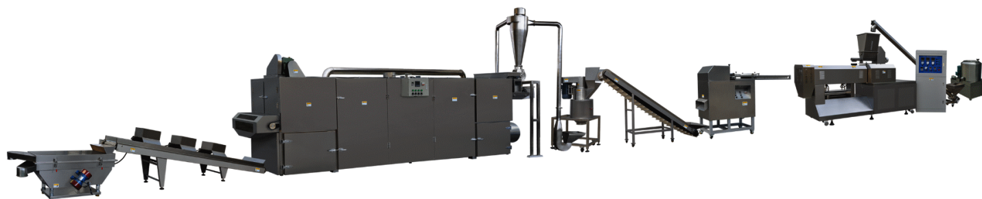
Flow Chart of Bread Crumbs Making Machinery
