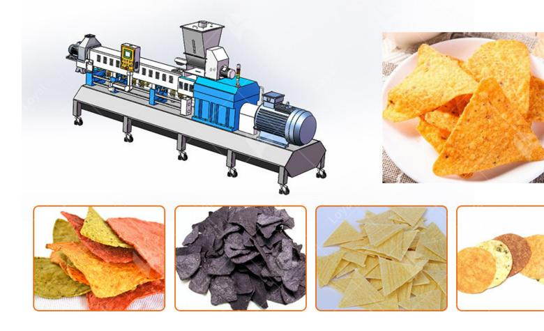
The Flowchart Of Baking Doritos Corn Chips Process Line 1.Flour Mixer --- 2. Screw Conveyor --- 3. Double Screw Extruder --- 4. Shaping Machine --- 5. Cooler ---Baking Machine --- 7. Flavoring Line
