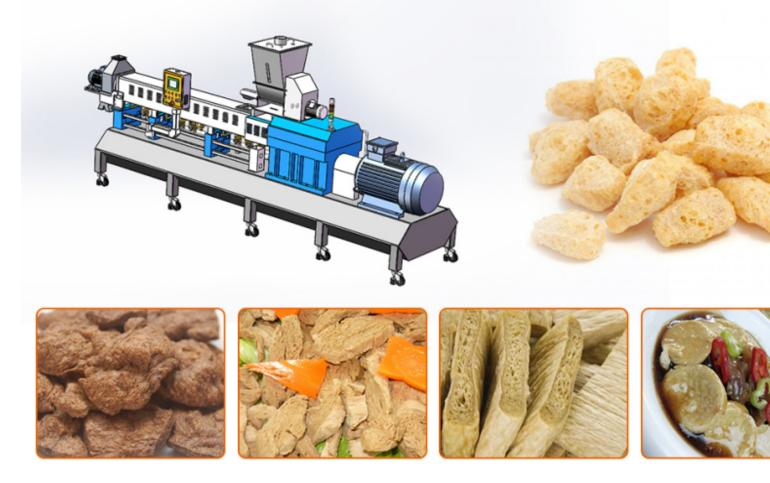
The whole Textured Soya Protein production line can automatically complete the production from mi extruding, air conveyor, multi-layer oven, cooling conveyor to the finished product.
