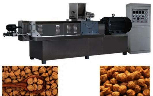
The **Soya Meat Making Machine** is highly automated, and the process is relatively simple. A whole production line comes down to complete the production of soy meat. By changing different molds, it can also produce other types of food, such as vegetarian steak, vegetarian chicken wings, vegetarian meat, vegetarian chicken, bean shrimp, bean sausage, etc. It greatly saves labor time, improves work efficiency, and has many advantages.
