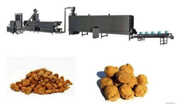
Soybean meat production line consists of mixer, screw conveyor, twin-screw extruder, airflow convey elevator, seasoning roller oil sprayer, cooler, packaging machine. The working conditions of the main equipment are as follows:
