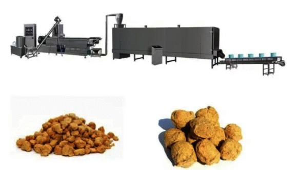
Soybean meat production line consists of mixer, screw conveyor, twin-screw extruder, airflow conveyor, dryer, elevator, seasoning roller oil sprayer, cooler, packaging machine. **The working conditions of the main equipment are as follows:**
