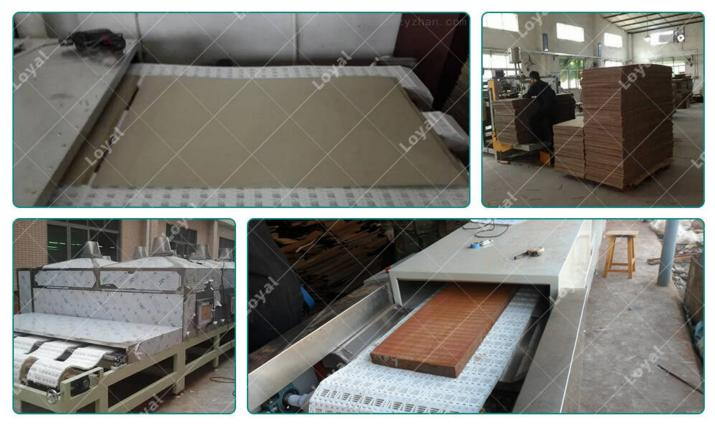
Test of Industrial Tunnel Sawdust Paper Cardboard Microwave Drying Machine in Customer's Workshop
