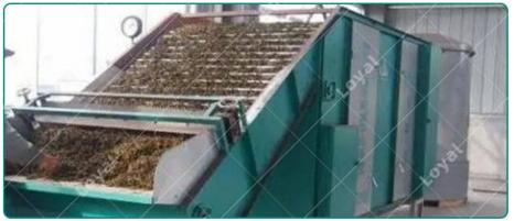
**Test of Herbs Leaves Tea Industrial Belt Type Microwave Dryer Microwave Drying Machine in Customer's Factory**
