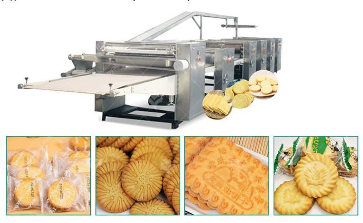
Trough toughening, crisp type forming machine, can produce hard biscuit, cake buscuit, walnut cake biscuits, thickness can be adjusted, and mechanical operation, frequency control of motor speed, adjust freely according to different products, and has advanced functions such as leakage power and alarm automatically. Automatic temperature adjustment freely according to different products, baking, automatic transmission, automatic fuel injection, automatic cooling, etc.
