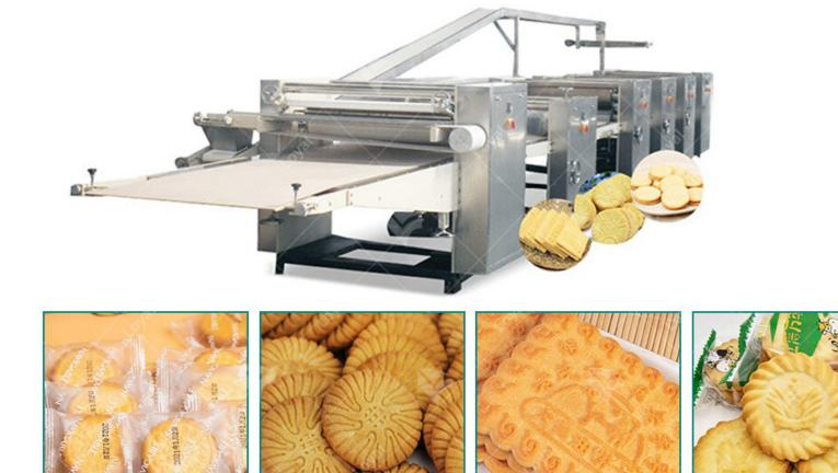
Trough toughening, crisp type forming machine, can produce hard biscuit, cake buscuit, walnut cake biscuits, thickness can be adjusted, and mechanical operation, frequency control of motor speed, adju according to different products, and has advanced functions such as leakage power and alarm automatically. Automatic temperature adjustment freely according to different products, baking, autor transmission, automatic fuel injection, automatic cooling, etc.
