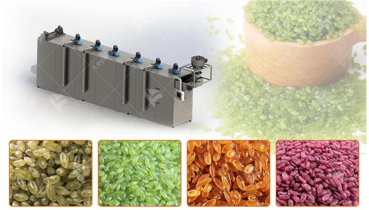
The line can use rice, millet, black rice and buckwheat as the main raw materials. Then it can be treated with vitamins, proteins and mineral substances. After the process of extrusion, steaming and forming, it can make fortified rice, golden rice, buckwheat rice, etc. The steaming method is the same as that of natural rice. Cooking is the same as natural rice, or even easier and more convenient.
