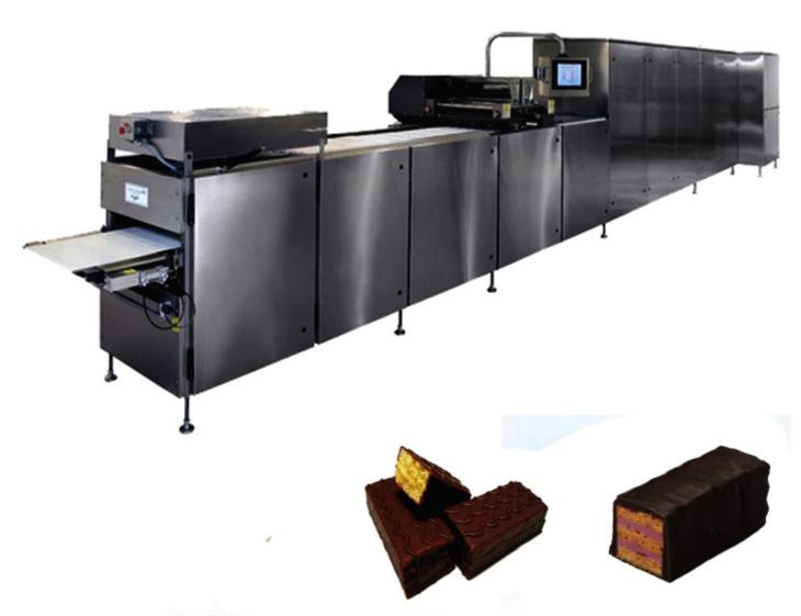
The ingredients are first mixed according to the cookie recipe, fed into the mixer, and the appropriate amount of milk or water is added to mix the ingredients and knead them into a smooth dough. The kneaded dough is fed into the cookie forming machine, where it is first rolled into cakes and then cut into fixed shapes, which can be produced in many different shapes, including round, square, figure, and flower shapes, by simply changing the mold.
