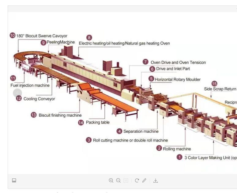
Equipment List of Hard BiscuitProduction Line dough mixer?compound rolling and shaping machine?oven?oilsprayer?cooling machine?sorting machine?packaging machine
