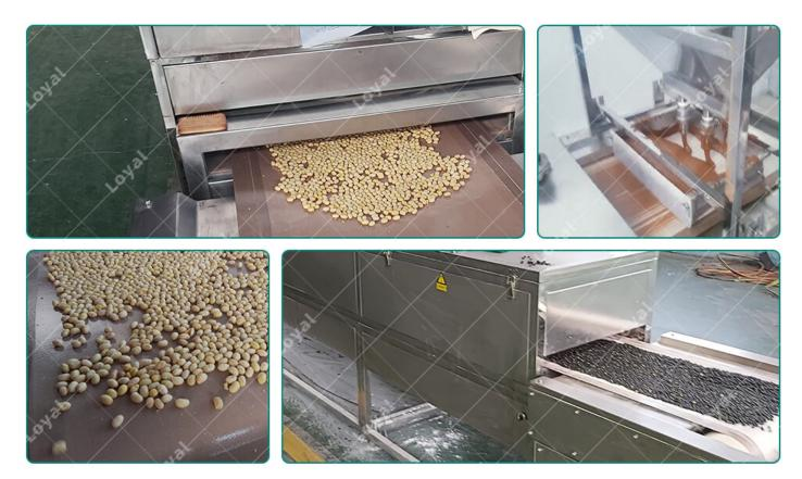
**3. Microwave sterilization,** preservation is the result of the combined effect of microwave thermal and non-thermal effects. Therefore, microwave sterilization temperature is lower than conventional methods, in general, the conventional method sterilization temperature to 120 ? -130 ?, about 1 hour, while the microwave sterilization temperature of only 70 ? -105 ?, about 90-180 seconds.
