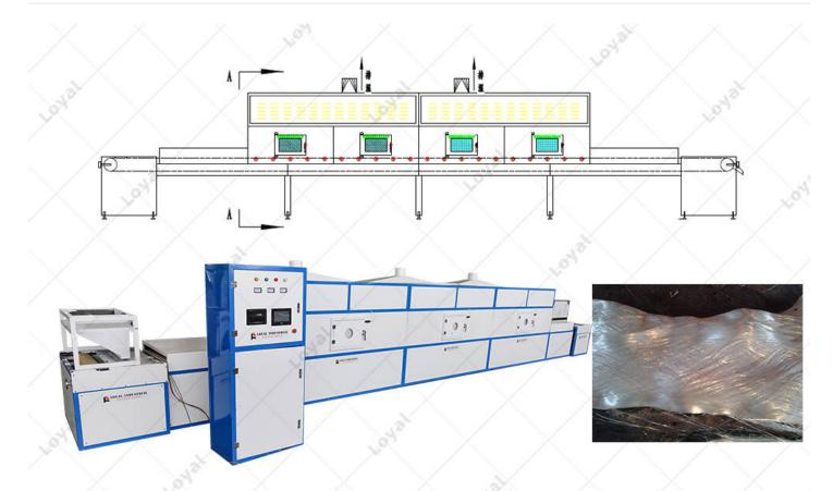
CAD High Efficient Industrial Microwave Glass Fiber Drying Machine Microwave Glass Fiber Drying Oven
