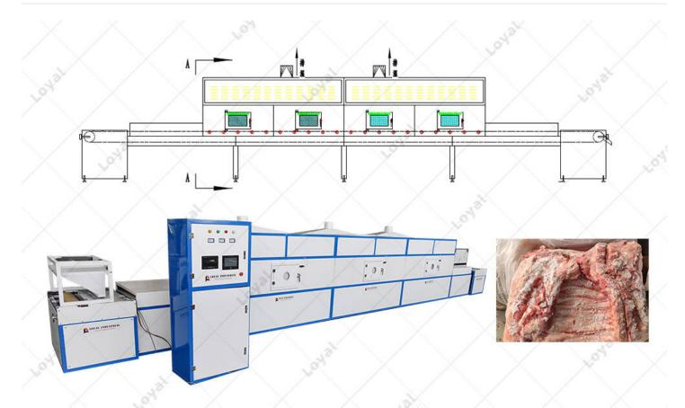
CAD of Tunnel Microwave Frozen Meat Mutton Processing Thawing Machine **What Is The Applications Of The Tunnel Microwave Thawing Machine?** Microwave frozen product thawing equipment is mainly used for rapid thawing of meat or non-meat frozen products such as seafood, aquatic food, chicken meat, pork meat, beef, mutton, fruit and other agricultural products.
