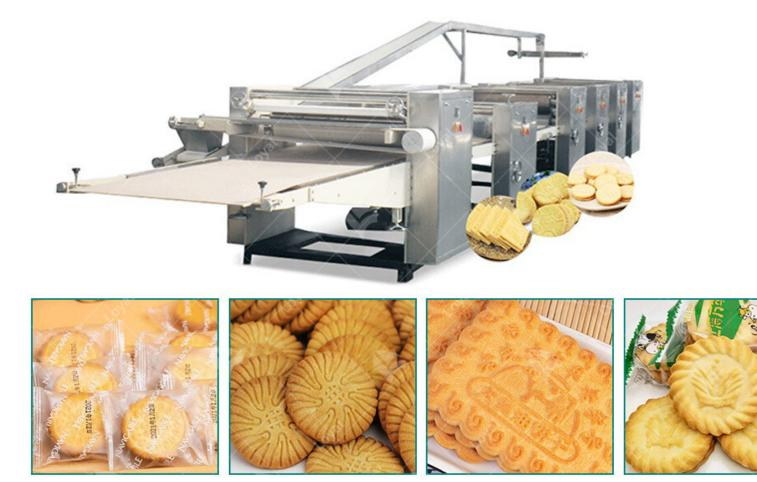
Trough toughening, crisp type forming machine, can produce hard biscuit, cake buscuit, walnut cake biscuits, thickness can be adjusted, and mechanical operation, frequency control of motor speed, adju according to different products, and has advanced functions such as leakage power and alarm automatically. Automatic temperature adjustment freely according to different products, baking, autor transmission, automatic fuel injection, automatic cooling, etc.
