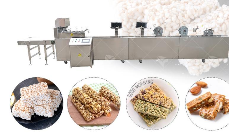
This production line has the advantages of more machines choice,flexible and diverse configurations range of raw material application, numerous in products variety and easy operation. The shapes of constant can be round, cylindrical, square, semi round, triangular and blossom etc.
