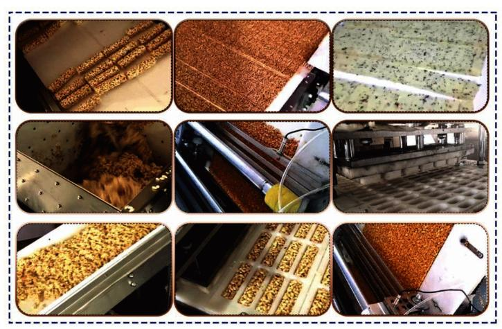
**Detailed Main Equipment Picture Of Candy Fruit Energy Granola Bar Line** Breakfast peanut chikki candy fruit energy granola bar making machine adopts PLC operating system and advanced mechanical structure to realize fully automated Production. The chocolate granola bar making line continuous feeding, automatic flattening, automatic cutting and cross-cutting. Compared with traditional hand-made methods, the cereal bar machine reduces a lot of production costs and improves production efficiency.
