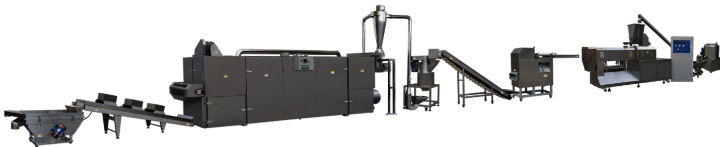
Flow Chart of Bread Crumbs Processing Line
