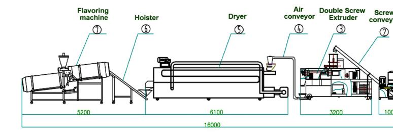
Flour Mixer-Screw Hoister-Double Screw Extruder-Hoister-Oven-Cooling Conveyor-Packing Machine
