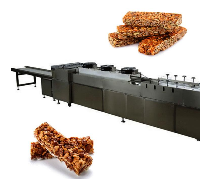
In the actual production process, the workers only need to select some high-quality raw materials, pr them. Then boil various sugars and some food additives in the boiling sugar pot according to the reci make the binder, and then mix the pretreated cereals with the binder in the mixer.
